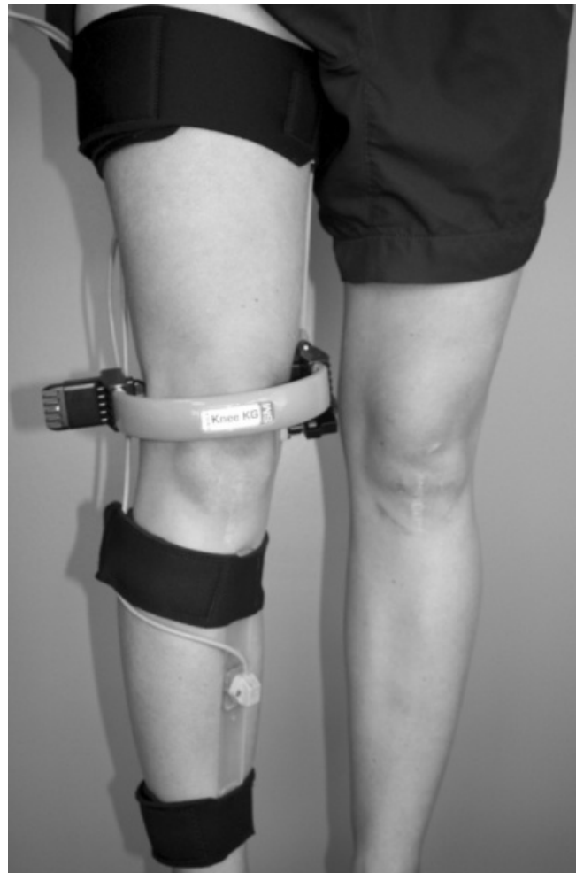
Figure 2. Attachment system developed and validated by the Imaging and Orthopaedics Laboratory, University of Montreal Hospital Centre, Montreal, Quebec, Canada. Semi-circular rigid ring is affixed between medial and lateral femoral condyle and tracks the 3D displacement of the femoral segment, whereas a semi-rigid plastic sheet is fixed along the longitudinal tibial axis and tracks the tibial segment [8, 10, 11].
